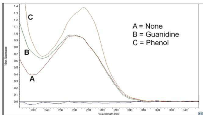
Although the spectra cannot diagnose problems *per se*, examination may assist in identifying that a problem exists and in narrowing down the source of the problem. Many contaminants absorb at around 230 nm or less; many of these create problems with downstream applications. In addition to examining the 260/280 ratio and the general shape of the spectra, we recommend the following:
