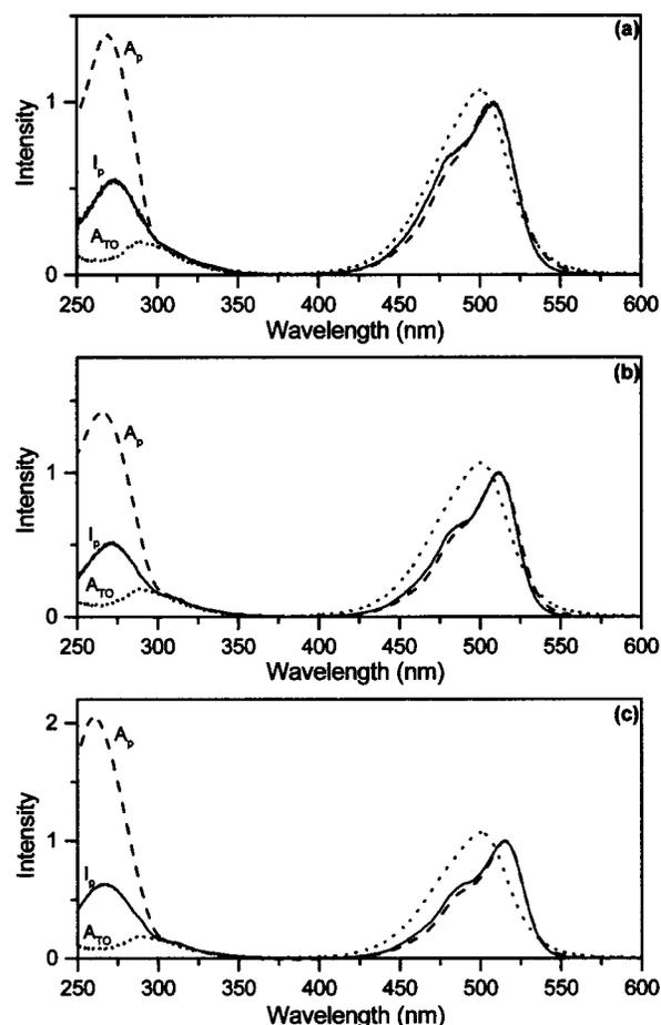
**Figure 2.** Absorption,  $A_p$ , (---) and fluorescence excitation,  $I_p$ , (—) spectra of (a) pyr-LUP, (b) AG-LUP, and (c) mix-LUP recorded at 15 °C. The absorption spectrum of free TO,  $A_{TO}$ , is shown for comparison (···). The spectra are normalized to have the same area in the interval 300–350 nm.
