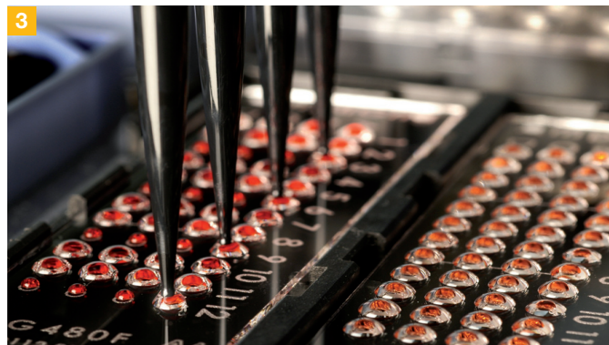
Automation of 1 µl AmpliGrid AG480F amplification reaction on Hamilton MICROLAB STAR ET , SW version 4.1
