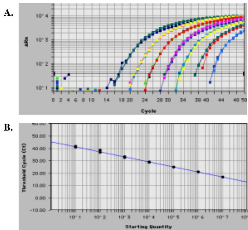
**Figure 2:** Real-time fluorescence measurements during PCR amplification, using the Amplifluor™ Universal System on ABI 7700. A. Threshold cycle (Ct) values were calculated from the amplification plot for 10<sup>1</sup> to 10<sup>7</sup> target copies of *bcl-2*. B. When plotted as threshold cycle (Ct) versus the input amount of target, the resulting standard curve is linear >5 orders of magnitude. The correlation coefficient ( $r^2$ ) is 0.998.
