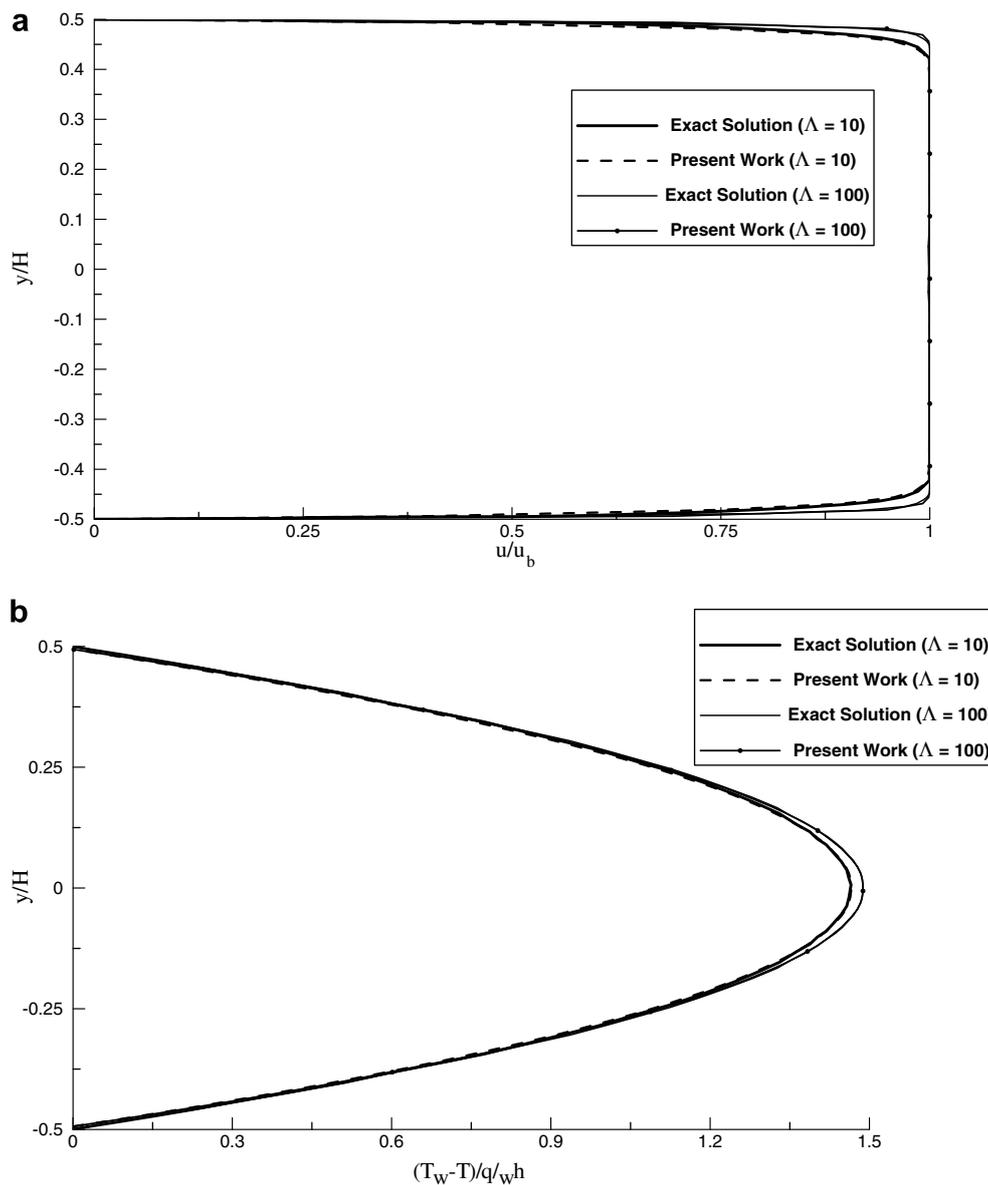
Fig. 2. Comparison of the present work with an exact solution [44] at the midsection of a channel filled with a porous medium (a) dimensionless velocity profile at  $Da^{-1/2} = 30$ ,  $\Lambda = 10, 100$  (b) dimensionless temperature profile at  $Da^{-1/2} = 30$ ,  $\Lambda = 10, 100$ .
