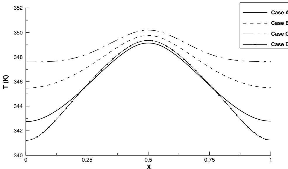
Fig. 6. The effects of exit channel thickness and location on the temperature distribution at the silicon–glass interface at  $t = 0.02$  s.
