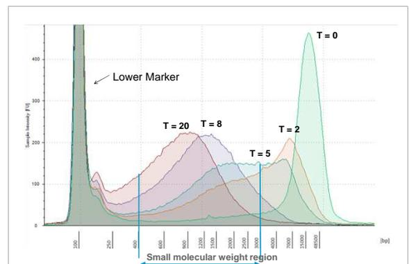
Figure 8: Electropherogram overlay of genomic DNA (T = sonication time in minutes)
