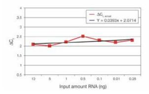
Figure 25. Relative efficiency plot. The  $\Delta C_1$  ranges from 2.0 to 2.5. When plotted against dilution or input amount of RNA, a slope is obtained. While a perfectly flat line (slope = 0) indicates identical efficiency across all input concentrations, a slope of <0.1 is generally considered acceptable when employing the  $\Delta \Delta C_1$  method.
