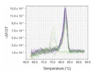
Figure 12. Melting curve analysis can detect the presence of nonspecific products, such as primer-dimer, as shown by the additional peaks to the left of the peak for the amplified product in the melt curve.
