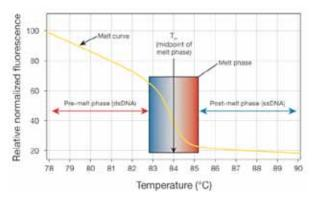
Figure 27. Characteristics of the melt curve profile for a PCR amplicon. Specific DNA sequences have characteristic melt-curve profiles. Mutations can be detected as either a shift in  $T_m$  or a change in shape of the melt curve. In contrast to traditional melt curve analysis, HRM can distinguish between amplicons with just a single-nucleotide difference. This technique has opened the door to many new applications for dsDNA-binding dyes.
