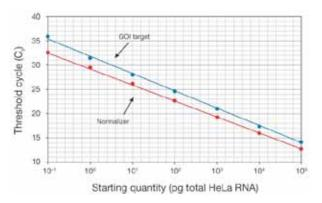
Figure 26. Efficiency values are obtained from standard curves to adjust the normalizer and gene-of-interest  $C_t$  values. HeLa RNA was diluted over 6 orders of magnitude, and real-time PCR was performed to generate standard curves for both the normalizer and gene of interest (GOI).
