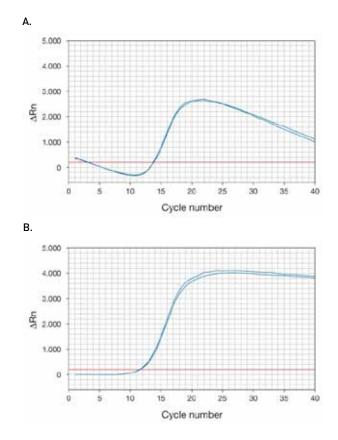
Figure 31. Amplification plots showing an incorrectly set baseline (A) and a correctly set baseline (B).
