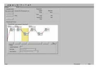
Figure 13. Example of a melting curve thermal profile setup on an Applied Biosystems<sup>®</sup> instrument (rapid heating to 94°C to denature the DNA, followed by cooling to 60°C).
