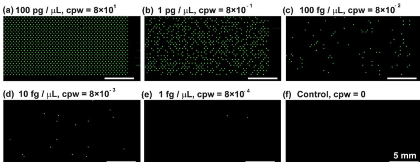
**Fig. 3** Digital PCR on the SlipChip with different concentrations of *S. aureus* gDNA. (a–e) Digital PCR on the Slipchip with a serial dilution of target DNA template ranging from 100 pg  $\mu\text{L}^{-1}$  to 1 fg  $\mu\text{L}^{-1}$ . Concentrations of gDNA and expected copies per well (cpw) are indicated above each figure. (f) Control, no wells showed positive signal when no target DNA template was loaded.
